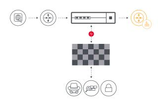
**Context-Aware Data Processing** - To get the right data to the right security tools, packet brokers use intelligent data processing to recognize rich metadata and deliver enhanced NetFlow information. This goes deeper than source and destination ports and IP addresses. Context-awareness requires a deep understanding of network
