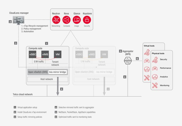
Figure 1. CloudLens deployment in an OpenStack / KVM environment
