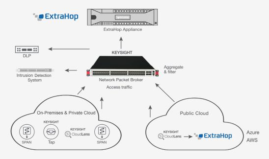
Keysight network packet brokers sit between access points in the network and ExtraHop appliances, aggregating and forwarding traffic from multiple taps and switched port analyzer (SPAN) ports to ExtraHop systems for analysis. This approach provides reliable, cost-efficient visibility for managing network and application performance across networks of any size.
