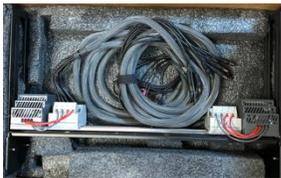
The Industrial power supply rack can support 48V DC or 110-220V AC input power, and support up to 32 x 5VDC powered devices. TAA Compliant, the 19" rack mount supports both AC and DC DIN mountable power supply convertors available separately from Keysight.
