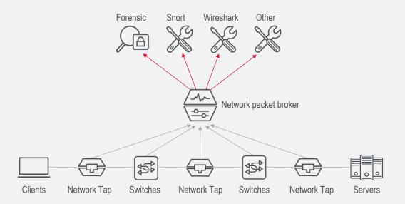
The simplest solution is to deploy a network packet broker (NPB) with taps. Taps provide a complete copy of data, which can then be optimized (e.g., filtering, deduplication, Secure Sockets Layer (SSL) decryption) by the NPB and distributed to the requisite monitoring tools.
