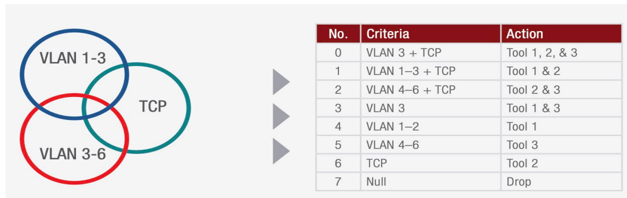
Figure 1. Example1- the right way to use priority filtering mode – complexity goes exponential when the number of rules or ports increase
