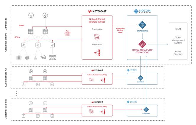
Note: other sites not shown here use Nozomi collectors to aggregate SPAN traffic
